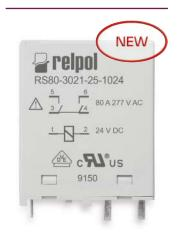
**③** To ensure proper operation of the relay, it is required to use multi-layer boards and make a connection on the PCB of pins 3-4 and also of pins 5-6.
