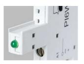
**Green LED**: signalling the operation status of the relay.
